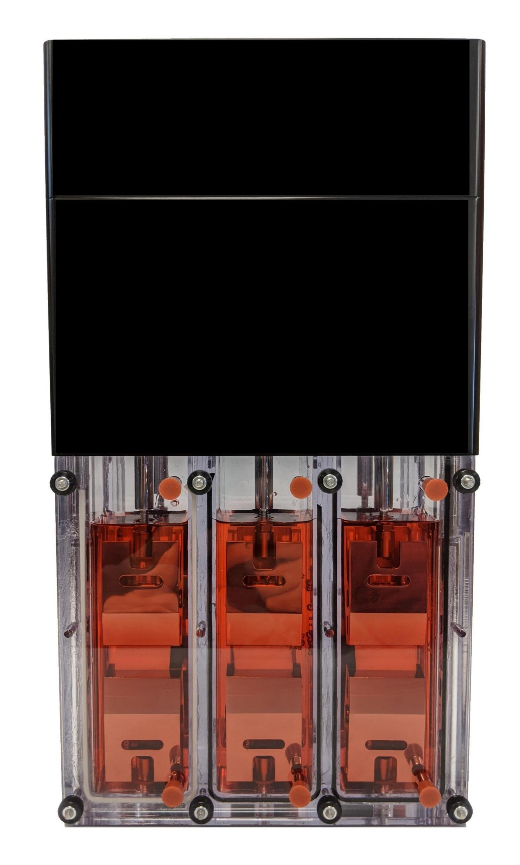
protocol. During the test, users can visually observe the specimens through the transparent chambers and measure changes in specimen stiffness. After the test, specimens can be removed for further macro- and micro-scale analysis.
