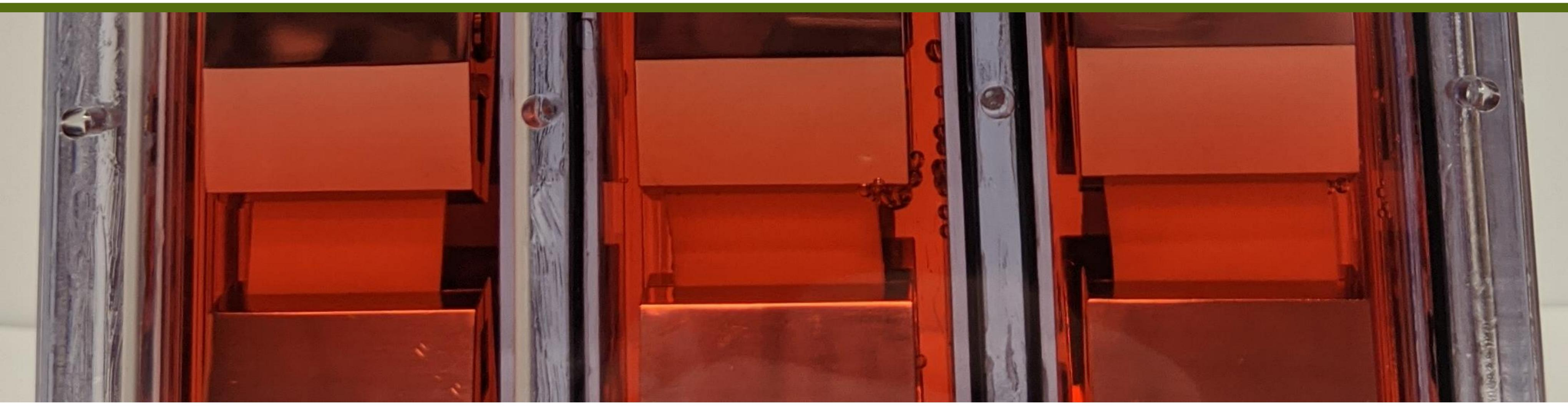
The MechanoCulture J1 is capable of running 6 cyclic mechanical stimulation tests on a variety of tissues, scaffolds, and constructs. Each test chamber is equipped with its own actuator and force sensor running an independent test
