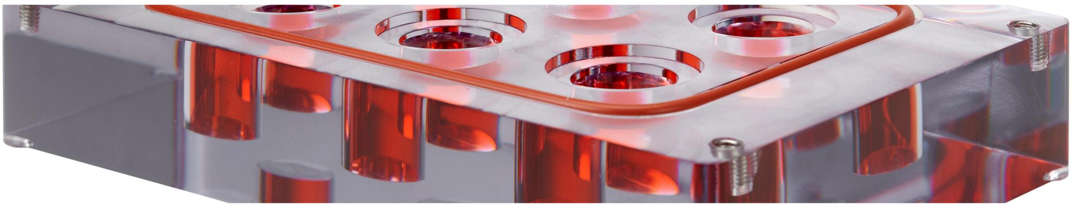
The **MechanoCulture TX** can be programmed to run constant velocity or sinusoidal compression patterns. Magnitudes, frequencies, rest periods, and cycle counts can all be specified in the accompanying software application and programmed to the device.
