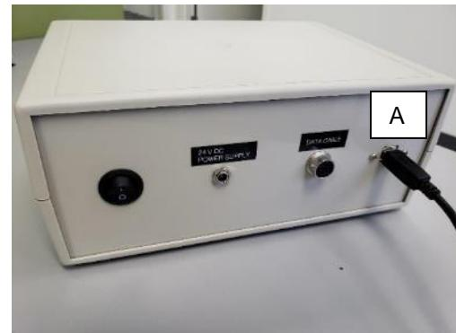
2. Connect the 24V DC power supply cable. Plug it into an appropriate 100-240V AC power source and the other end into the pressure regulator box.
