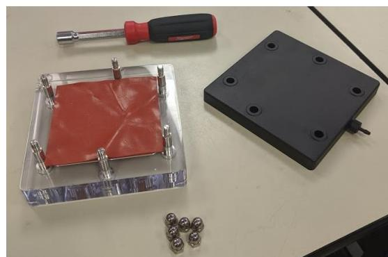
2. Remove the washers and lift the top cover off the specimen holder.
